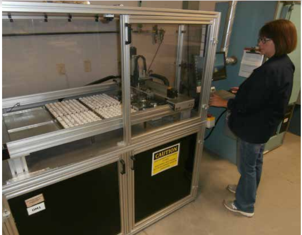
Modern soil analytical laboratories utilize robotic sample handling systems and the latest chemical analysis methods to provide accurate test results to golf course managers. Photo courtesy of Brookside Laboratories
