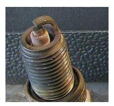
What does the condition of the insulator and electrode indicate?
