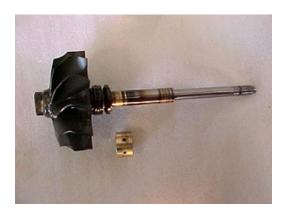
What is the likely cause of the excessive heat that produces the discoloration?
