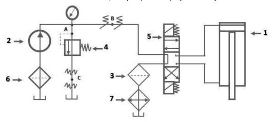
The pump relief is set at 2,500 psi (172 bar) and is running but the valve is not shifted.
