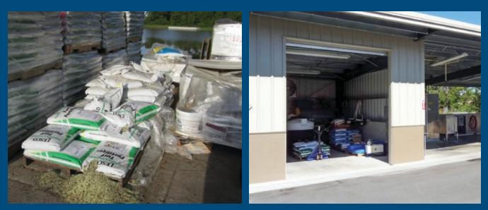
FIGURE 5.18: Fertilizer: left, no cover, open spills; right: good practices, inside storage
