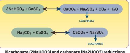
Bicarbonate (2NaHCO3) and carbonate (Na2HCO3) reductions following gypsum (CaSO4) application.
