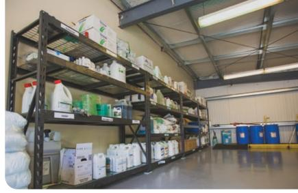
When designing the facility, keep in mind that temperature extremes during storage may reduce safety and affect pesticide efficacy. Provide appropriate exhaust ventilation and an emergency wash area. The emergency wash area should be located outside the storage building. Local fire and electrical codes may require explosion-proof lighting and fans. The light/fan switch should be located outside the building so that both are on before people enter and until they have left the building.
