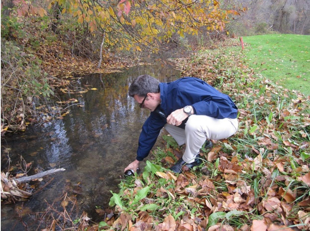
*Figure 8. Drawing a water sample.*
