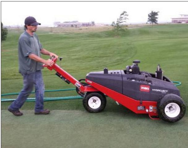
Figure 29. Getting water directly to the roots with a hydroject machine.
