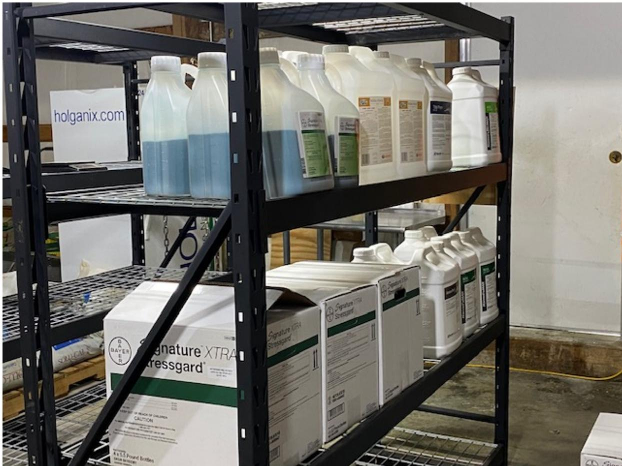
*Figure 19. Wood shelving should never be used, because it may absorb spilled pesticides. Metal should be painted to stop corrosion. Photo credit: Kevin Glover.*
