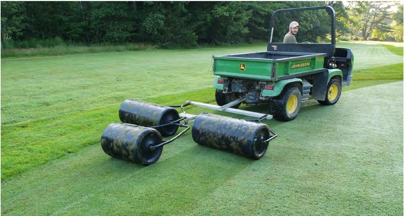
**Figure 6-7.** Rolling putting green surfaces can allow managers to reduce mowing frequency or raise mowing heights while maintaining putting green speeds.
