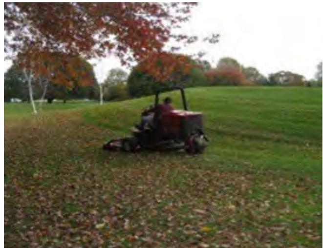
**Figure 6-4.** Rotary mowers are used for rough and surrounds (bunker, green, and tee). Sharp rotary blades are necessary for a quality cut and plant health. Photos from New England Regional Manual.
