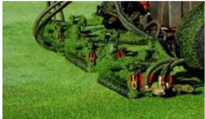
**Figure 6-3.** Reel mowers are used on greens, collars, tees, approaches, and fairways. Proper reel to bed knife adjustment is necessary to maintain plant health. Photos from New England Regional Manual.
