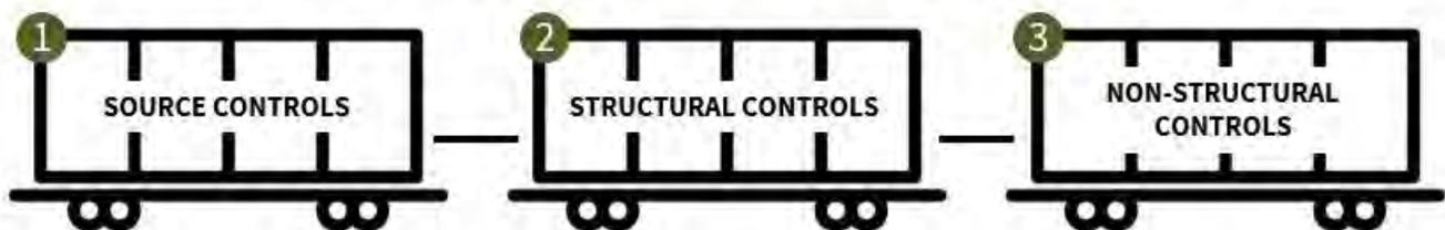
A stormwater treatment train directs stormwater runoff from one treatment to another by conveyance structures. Each ‘train’ provides treatment to the stormwater flowing through it. **1 Source controls** prevent the generation of polluted runoff, **2 structural controls** remove, filter, retain, or reroute potential contaminants, and **3 non-structural controls** mimic the natural hydrology before stormwater leaves the site.
