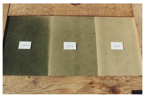
Figure 24. Sand particle application rate differences. Photo Credit: USGA.
