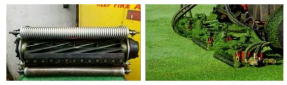
*Figure 6-3. Reel mowers are used on greens, collars, tees, approaches, and fairways. Proper reel to bed knife adjustment is necessary to maintain plant health. Photos obtained from the New England Manual.*
