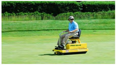
*Figure 6-7. Rolling putting green surfaces can allow managers to reduce mowing frequency or raise mowing heights while maintaining putting green speeds. Photo obtained from the New England Manual.*
