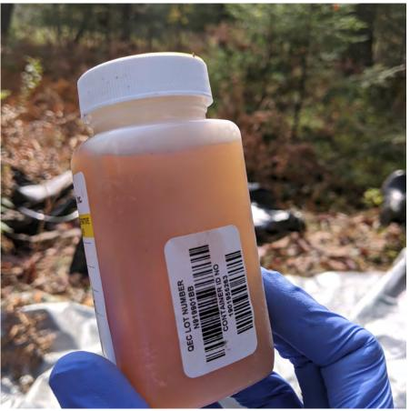
A visual inspection can indicate a contamination problem that is increasing turbidity of the water. © FBE.
