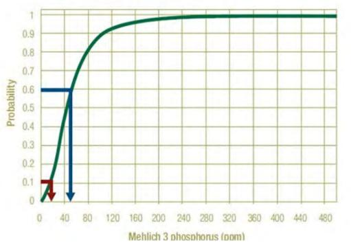
*Figure 5-3. The cumulative distribution function for phosphorus to identify the MLSN guideline. Figure obtained from New England Manual.*
