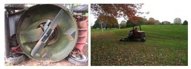
*Figure 6-4. Rotary mowers are used for rough and surrounds (bunker, green, and tee). Sharp rotary blades are necessary for a quality cut and plant health. Photos obtained from the New England Manual.*
