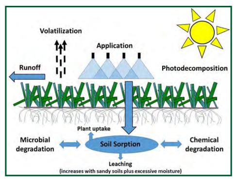
*Figure 8.3 Naturally occurring environmental processes causing pesticide dissipation. Figure obtained from New England Manual.*
