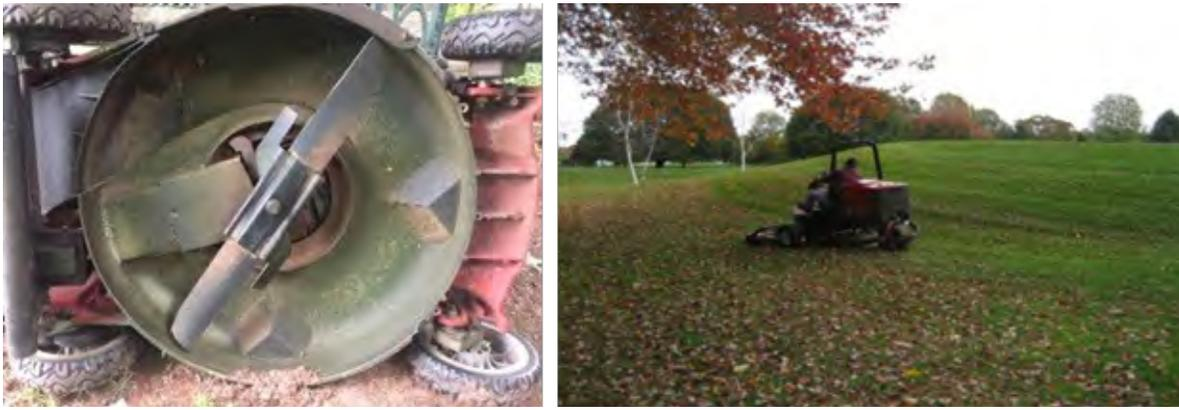
Figure 6-4. Rotary mowers are used for rough and surrounds (bunker, green, and tee). Sharp rotary blades are necessary for a quality cut and plant health. Photos obtained from the *New England Manual*.
