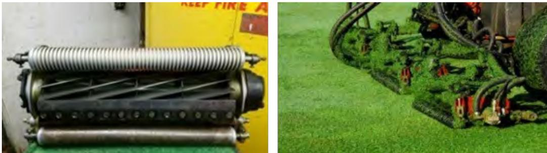
*Figure 6-3. Reel mowers are used on greens, collars, tees, approaches, and fairways. Proper reel to bed knife adjustment is necessary to maintain plant health. Photos obtained from the New England Manual.*
