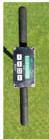
Figure 7. Soil moisture sensor.
