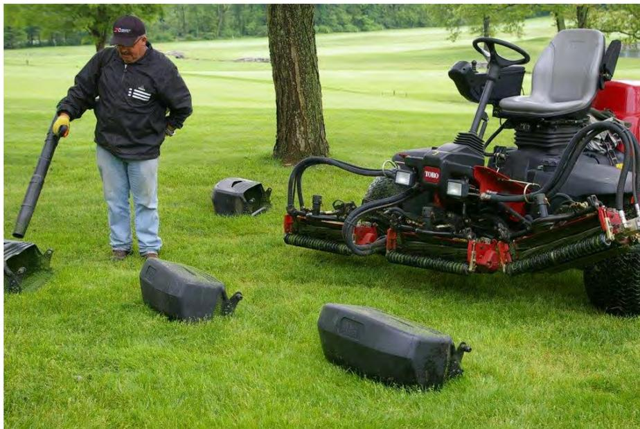
*Figure 31. Blowing clippings off equipment prior to washing.*
