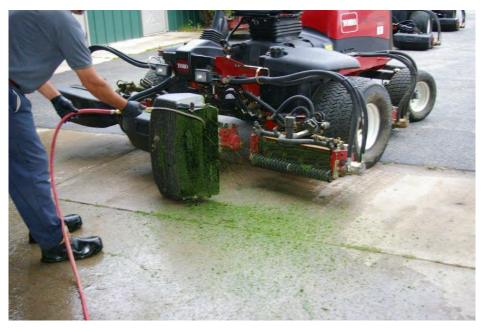
Figure 32. Equipment prewash on clippings collection pad.
