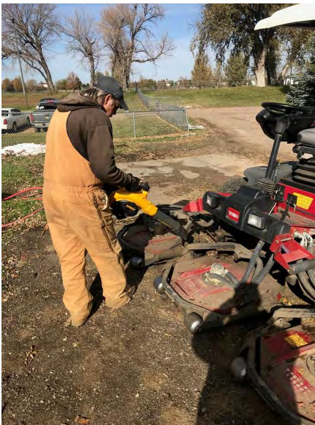
Figure 24. Using compressed air to blow clippings off mowers before washing can help reduce the amount of nutrients that enter drains via washwater.
