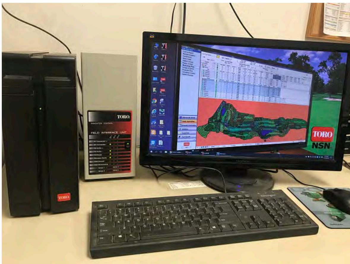
*Figure 12. Advanced irrigation control systems provide precision control and monitoring.*
