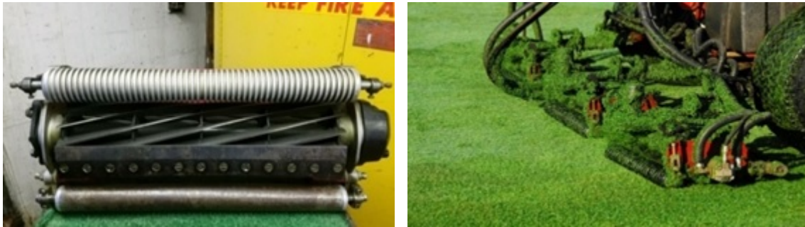
Figure 6-3. Reel mowers are used on greens, collars, tees, approaches, and fairways. Proper reel to bed knife adjustment is necessary to maintain plant health.
