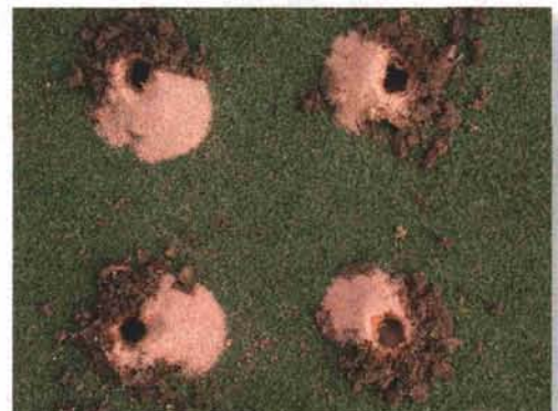
After the holes were drilled and the cores removed, the holes were filled with the amendment mixture. A mixture of 25% Profile and 75% sand (by volume) is shown here.
