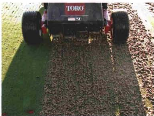
This greens aerator has been retrofitted with tine adapters allowing for a tine spacing of 1.25 x 1.5 inches.
