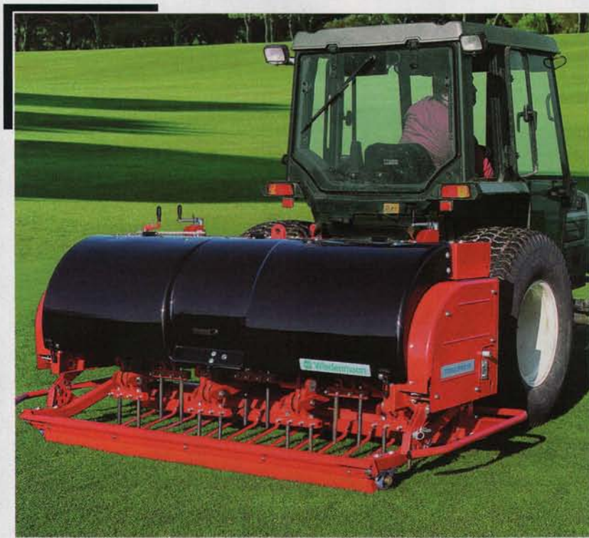
Deep-tine aerification promotes a deeper root system and allows superintendents to lengthen irrigation intervals. Photo courtesy of Wiedenmann Ltd.
