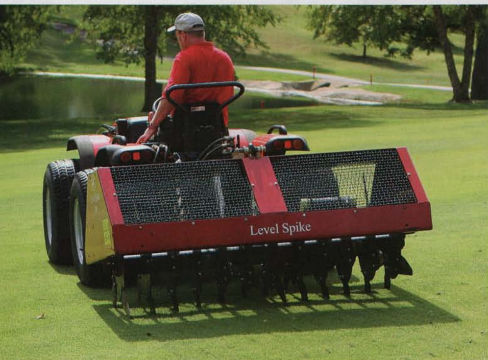
Use a combination of knives and spoon tines to aerate and improve drainage. Photo by Seth Jones
