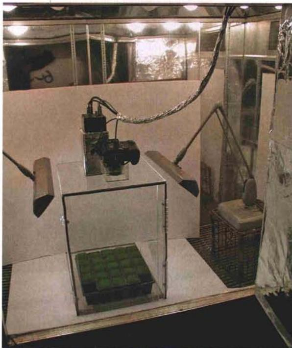
**Above:** The Plexiglas humidifier is contained in a growth chamber. Image-capturing devices are mounted 15 inches (38 centimeters) above the grass canopies and capture images simultaneously throughout the experiments.
