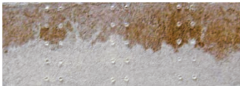
Top: Hydrophobic soil treated with a wetting agent. Note the uniform wetting front. Bottom: Hydrophobic soil profile not treated with a wetting agent. Note the nonuniform wetting. Photos by K. Tucker
