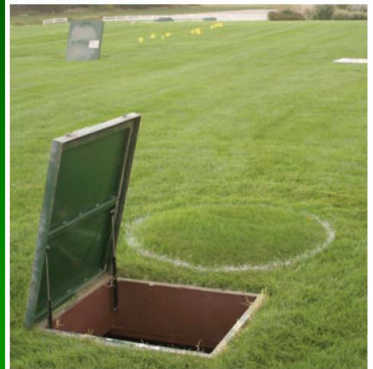
Since the summer of 1998, percolate samples have been collected from the same monolith lysimeters and analyzed for nitrate-nitrogen (NO 3 -N).
