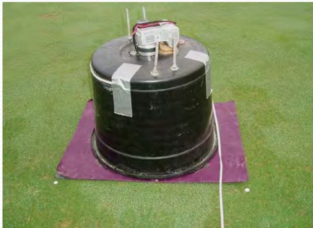
Light box with frame marked by two golf tees at corner to assist in finding ball marks
