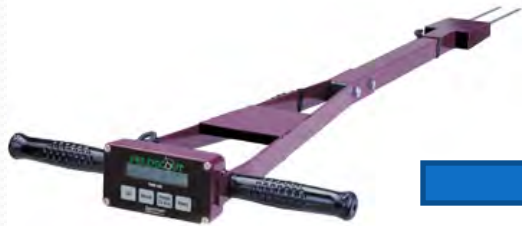
FieldScout 300 TDR Soil Moisture Meter (Spectrum Technologies) with 3.8 cm (1.5 inch) probes
