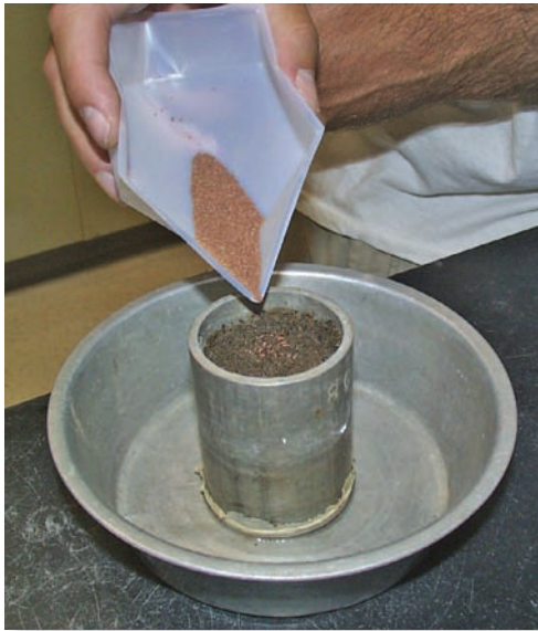
Ash produced from the fertilizers was applied to cylinders containing a USGA-specified root-zone mix at rates equal to the amount that would be applied when using that product to deliver 5, 10 or 20 pounds of nitrogen/1,000 square feet (24.4, 48.8 or 97.6 grams/square meter). Photos by A. McNitt
