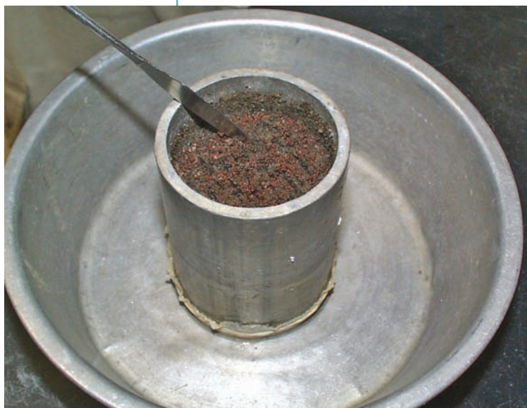
Three replications of each treatment were performed where the ash was applied to the surface of the root zone in the cylinder before compaction, and three more replications were performed where the ash was applied to the surface and worked into the top 0.16 inch (4 millimeters), as shown in the photo.
