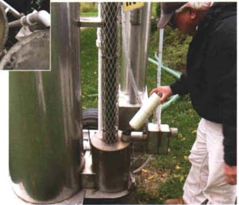
Jeff's portable sulfur burner on wheels.
